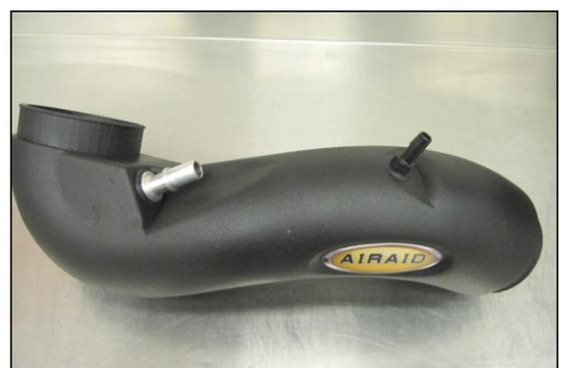
6. A.) Install the 3/8" Barbed Fitting (#5) into the threaded hole in the Intake Tube.
