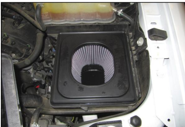
4. Install The Airaid Premium Filter (#1) into the airbox.
